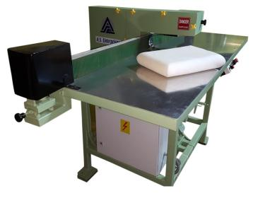
The table is adjustable in height with respect to the blade.
